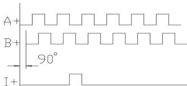
Differential signals will have additional channels A<sup>-</sup>, B<sup>-</sup>, I<sup>-</sup>.
